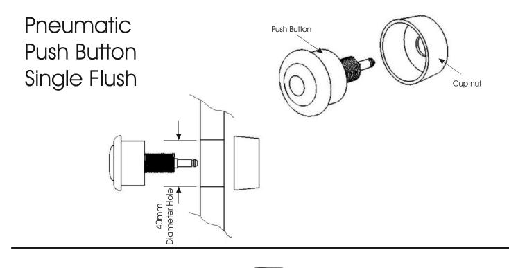
Pneumatic Single Flush Outlet Valve
